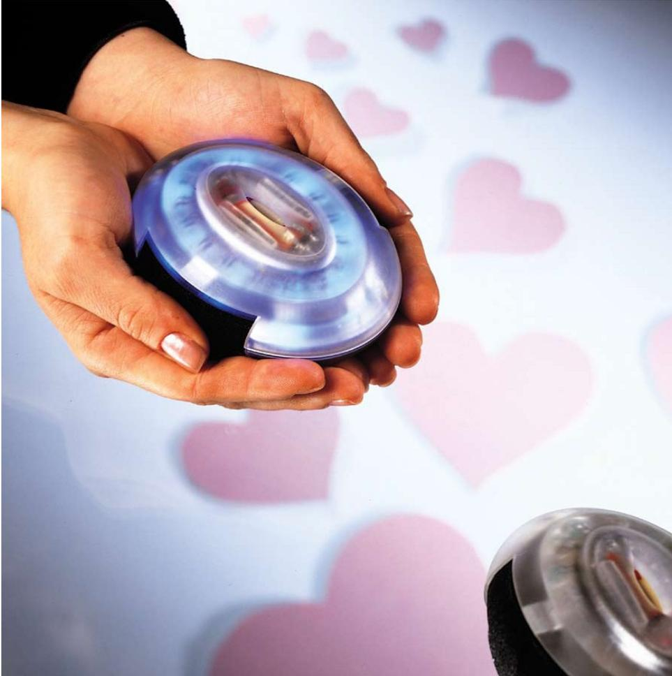
The **Kiss Communicator** is a concept prototype that allows you to blow a .kiss. to your beloved even when in another part of the world. Squeezing and blowing on the device wirelessly sends a sequence of lights to its corresponding Communicator. (p. 53)
