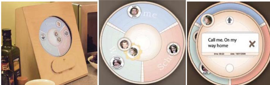
The **Whereabouts Clock**: the lefthand image shows the clock in its case; the middle image is a close-up of its interface; and the righthand image shows what happens when you touch on a text message. (p. 71)
