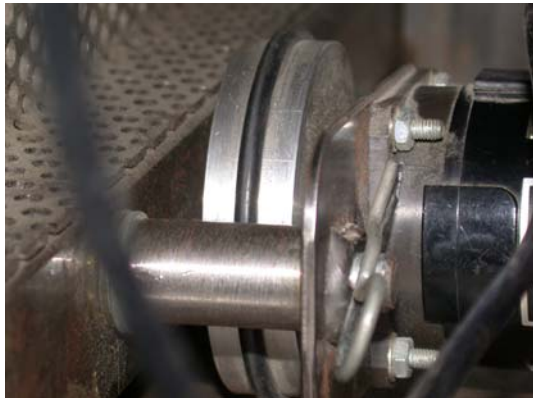
Close-up of the tracking wheel/optical encoder
