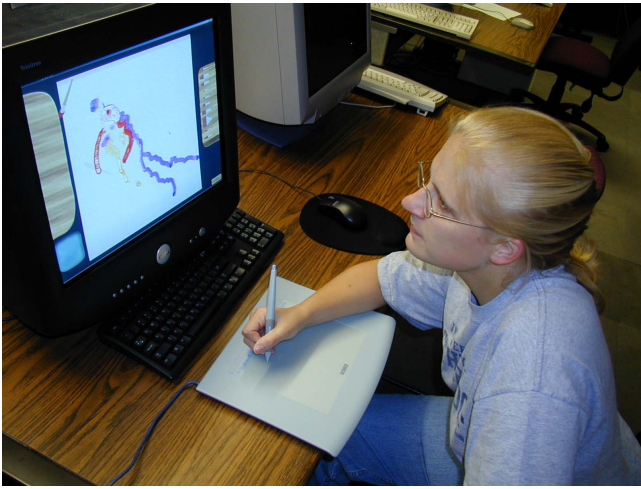
Figure 2: The physical system setup with a tablet interface. We use the Wacom Intuos2 line of tablets which reports stylus X-Y tilt as well as pressure and X-Y location. From these 5 measurements we derive a 3D transform for the brush. We also support the Phantom haptic input device.
