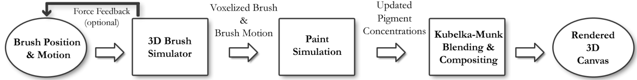
Figure 3: System Architecture. We start with input from either a pressure- and tilt-sensitive tablet or Phantom haptic IO device, then simulate the brush, simulate the paint, and render the painting’s pigment concentrations into a final RGB image for display. Fig. 5 details the 3D Paint Simulation stage further, and Fig. 6 shows the details of the K-M Rendering stage.
